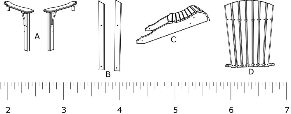
1. Attach (A) Armrest Assembly to (C) Seat Assembly Using 2 - 3" Wafer Bolts per side, Tighten Wafer Bolts with included Hex Key, Be sure to match all numbers & or letters.
