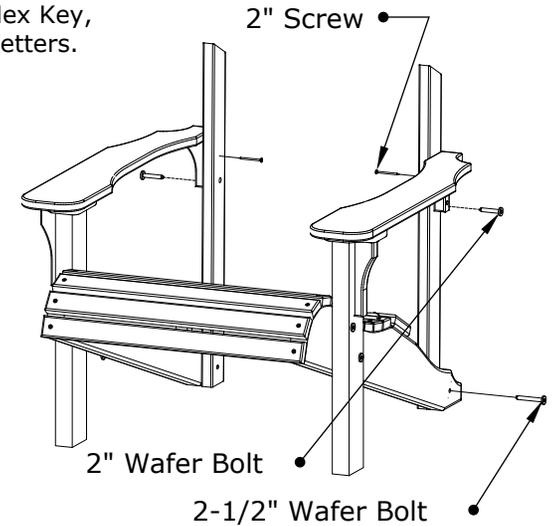
3. Attach (D) Back Assembly to (B) Back Legs & (C) Seat Assembly using 4 - 2" Screws per side, be sure to match all numbers & or letters.
