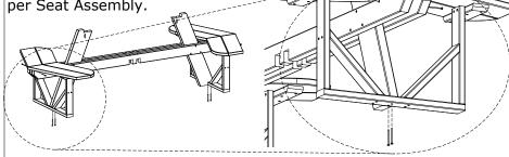
3. Set together both Leg Assemblies installing 4 - 2 1/2" Screws .
